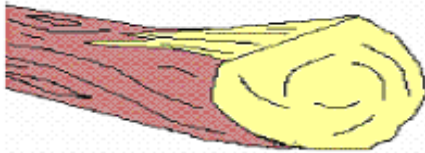
Shatter confined to flare OK
